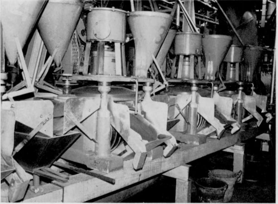
Fig. 7. — Berjantai Tin Dredging's tin shed (McLean Magnetic Separators).
